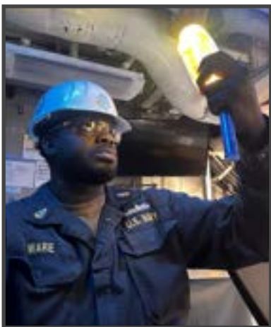
GSMC (SW) Michael Ware, conducting a clear and bright test on a fuel sample. (Photo by Steven Constantino.)
