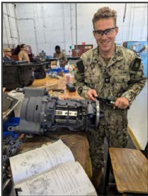
FC2 Samuel Bach installs the end plate coupler on the rear housing of a close-in weapon system. (Photo by FC1(SW/AW) Bryan Dewanz.)
