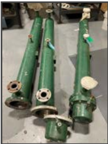
Ship Service Turbine Generator (SSTG) lube oil coolers sent to MARMC to be cleaned and refurbished. (Photo by MMN1(SW) Shane Diaz.)
