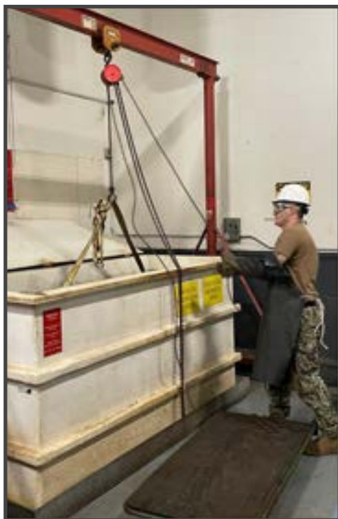
MMN1(SW) Michael Schell gently lowers a tube bundle into an acid bath to descale the tubes inside and out. Heat exchanger tube bundle have a lot of surface area by design, so chemical dips are the only effective way of thoroughly cleaning the bundle. (Photo by MMN1(SW) Shane Diaz.)
