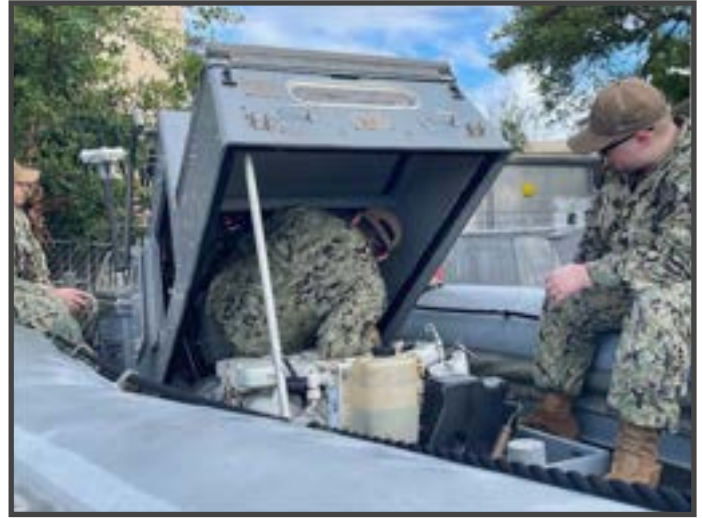
EM2 Declan Johnson (Left), EM2 Jayden Yeager (Center), and EM2 Matthew Rooney conducting a reference check of electrical circuit of a Rigid Hull Inflatable Boat. (Photo by MM1 (SW/AW) Logan Platt.)
