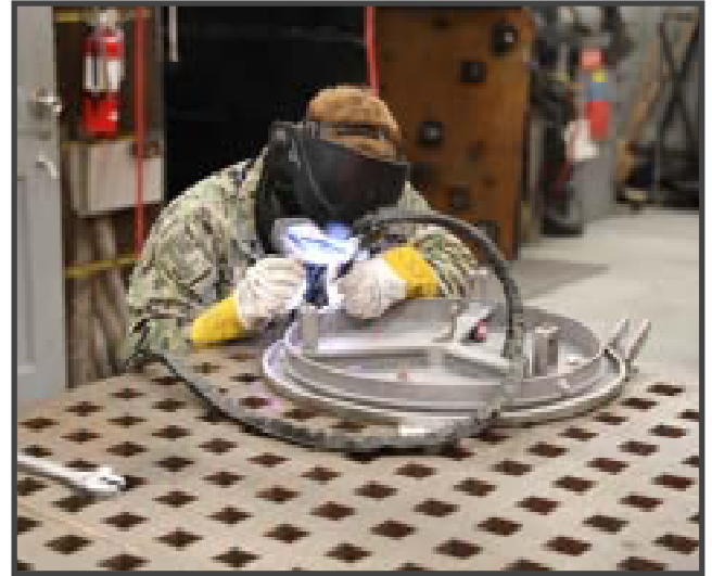
HT2(SW) Kenneth Woods, conducting weld repair on a scuttle for a destroyer. (Photo by MM2 (SW) Bianca Reiter, PAO.)
