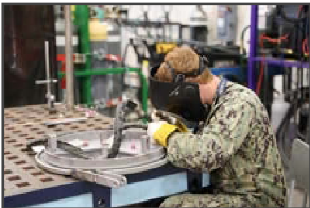
HT2(SW) Kenneth Woods, conducting weld repair on a scuttle for a destroyer. (Photo by MM2 (SW) Bianca Reiter, PAO.)
