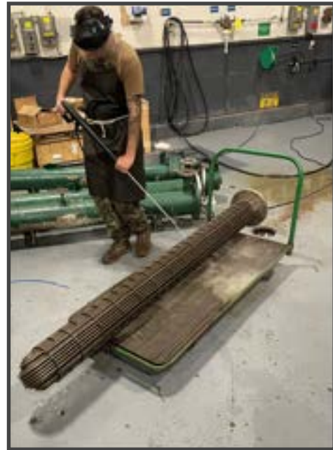
MMN1(SW) Michael Schell uses a pressure washer to remove any residual debris from the heat exchanger tube bundle after it has exited the acid bath. (Photo by MMN1(SW) Shane Diaz.)
