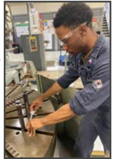
MR2(SW) Terry measures the distance between hold down bolts on a vertical turret lathe. (Photo by Rick Smith.)
