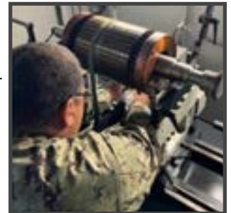
EM1 (SW) Joseph Naranjo working on balancing a rotor by taking measurements for equal weight distribution.
